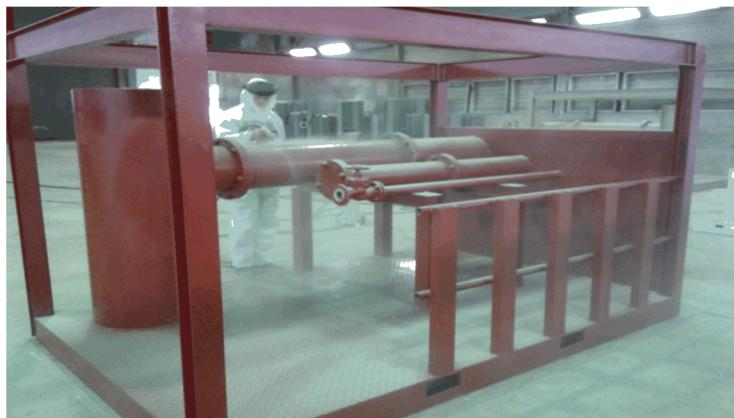
Dimensions of mist cloud (jet blasting on object (back side))
